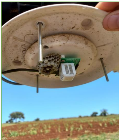
The Temp_RH sensor is inside the Gill Screens. Hornets make nests and frogs climb in there. This gives inaccurate temp and relative humidity readings.
