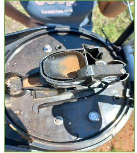
Sand, spiders or bugs on Rain bucket tippers. Cause inaccurate rain measurement. Unscrew Rain Bucket to clean this
