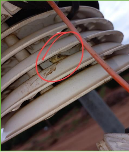
Frogs, Spiders and Hornets climb into the gill screens. This causes inaccurate Temp measurement
