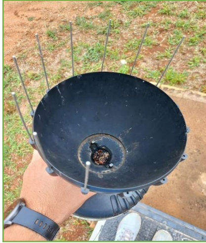
Rain Bucket blocked. Cause no rain measurement
